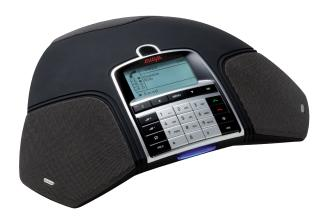
Superb sound quality: Avaya OmniSound® audio technology, unique to Avaya B100 Conference Phones, delivers crystal-clear voice transmission. A built-in, adjustable equalizer allows you get the sound levels just right. An omnidirectional microphone and three speakers all add to the optimal audio performance.
