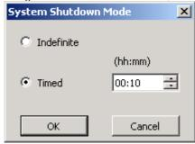
3. Select the type of shutdown required. If I ndefinite is used, the system can only be restarted by having its power switched off and then on again. If a Timed shutdown is selected, the IP Office will reboot after the set time has elapsed.
