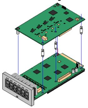
Most <u>IP500 base cards</u> scan be fitted with an IP500 trunk daughter cards to support the connection of trunks to the base card.
