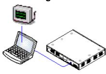
IP Office Monitor (also know as System Monitor) is a tool that can show all activity on the IP Office system in great detail. As a consequence, interpretation of Monitor traces requires a high-level of data and telephony protocol knowledge. However, all IP Office installers and maintainers must understand how to run Monitor when necessary as Avaya may request copies of Monitor traces to resolve support issues.
