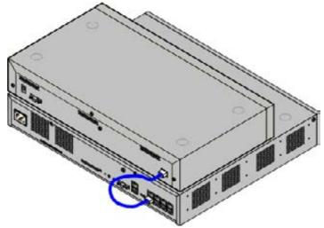
IP500 System with External Expansion Module
