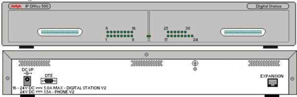
LEDs 1 to 16 or 1 to 30 indicate when a phone is connected. They do not indicate phone activity. The center LED indicate the module status (Green = Okay, Red = Error, Flashing = Loading firmware).
