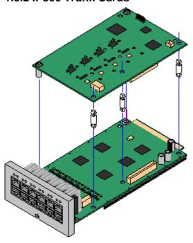
Most <u>IP500 base cards</u> 15 can be fitted with an IP500 trunk daughter cards to support the connection of trunks to the base card.
