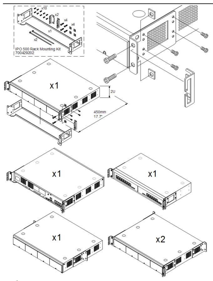
• 1 Only the screws provided with the mounting kit should used to attach the brackets to the control unit.
