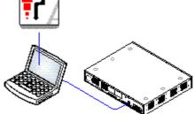
IP Office Manager is used to access all parts of the IP Office configuration. Manager can also be used to upgrade the software files used by an IP Office system.
