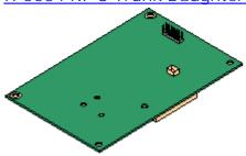
This card allows the base card to support up to 2 PRI trunk connections. The card is available in single and dual port variants. The card can be configured for E1 PRI, T1 robbed bit, T1 PRI or E1R2 PRI trunks
