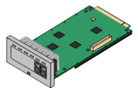
The maximum number of voice compression channels supported, using IP500 VCM base cards, Combination Cards and / or IP400 VCM cards on IP500 Legacy Card Carriers, is 148.
