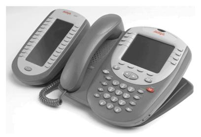
The EU24/EU24BL are phone expansion modules that work in association with a 5420, 5620/1, 2420, 4620/1, 4625 telephones. They provide an additional 24 programmable buttons with associated display label and status icons. Only one EU24 can be used per phone. The EU24BL has a backlight and is for use with the 4621 and 5621 only.
