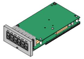
This card already includes an IP500 trunk card, therefore no additional trunk card is possible. A maximum of two of these cards is allowed in the chassis.
