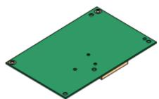
The ports on IP500 BRI cards can be individually configured to operate as an S-interface (S0 mode). When set as an S interface the settings for the Line will be exactly the same as for a circuit on an So8 Expansion Module.
