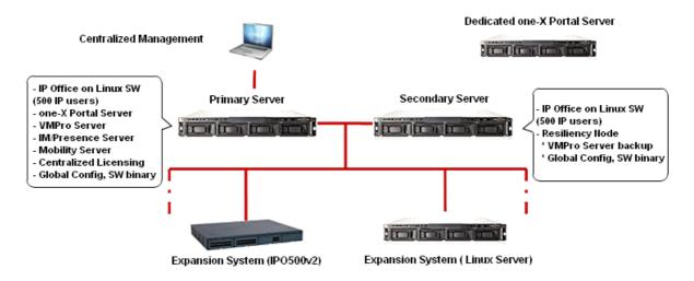
The Primary Server running the Avaya IP Office Server Edition Linux software is the main server and the only mandatory component required for the IP Office Mid-market offer to work. A secondary Linux server can be added for additional scalability and/or resiliency. The IP Office 500v2 expansion system can also be added for additional scalability or for adding support for analog/digital stations and trunk ports.
