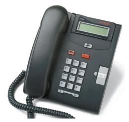
The T7100 telephone is part of the Business Series Terminals portfolio. It has one programmable button and a  $1 \times 16$  character alphanumeric display to provide call progress information. There are no display buttons (soft keys) on the T7100 and it does not support headset or Handsfree.
