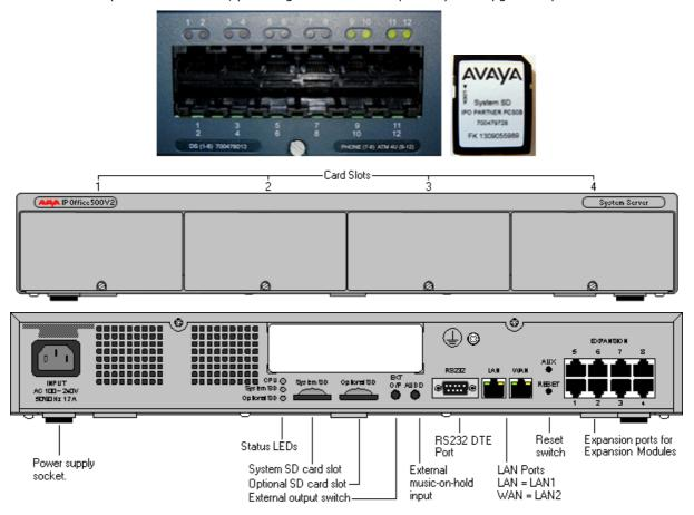
The front of the IP500 V2 Control Unit has 4 expansion bays, which supports the following system modules:
