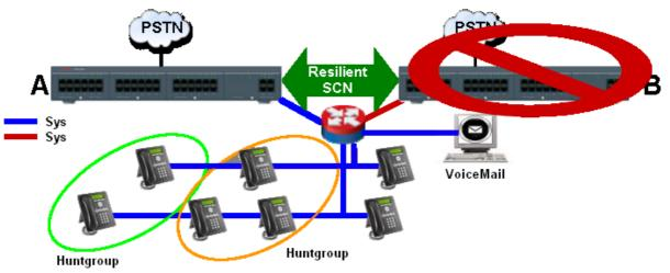
For Multi-Site Networks (SCN), VCM modules are required in all systems being connected. The IP lines may be configured in a start or a meshed configuration. One of the advantages of a meshed configuration is that it removes the risk of a single point of failure within the network. Also the names and numbers (groups, line, services, etc) on the separate IP Office systems should be unique to reduce potential maintenance confusion.
