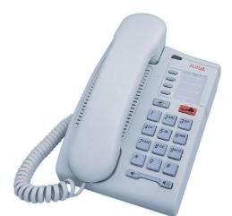
The T7000 telephone is an entry-level digital set for basic low-use office environments. It has four programmable feature keys. It does not have display buttons (soft keys), and it does not support headset or Handsfree.
