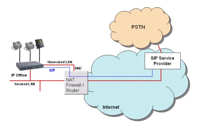
**Option 3:** Connection to the ITSP over NAT using 3<sup>rd</sup> party STUN (Simple Traversal of UDP through NAT) servers in the network to discover the NAT mechanism being used.
