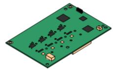
• When fitted to an IP500 Analog Phone 8 base card, the combination supports 1 power failure extension to trunk connection.
