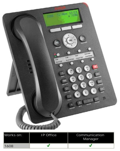
The Avaya 1608 supports 8 line appearances / feature keys. Each of the buttons includes dual LEDs (red, green) providing explicit status for the user. For a familiar look and feel, the 1608 includes several fixed feature keys for common telephone tasks including conference, transfer, drop, hold, and mute. In addition, the 1608 includes a high quality two-way speakerphone, and supports a broad portfolio of Avaya wired and wireless headsets through its integrated headset jack.
