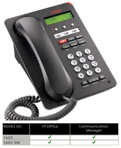
The Avaya 1603 supports 3 line appearances. Each of the buttons includes dual LEDs (red, green) providing explicit status for the user. For a familiar look and feel, the 1603 includes several fixed feature keys for common telephone tasks including conference, transfer, drop, hold, and mute. In addition, the 1603 includes a 2-way speakerphone. The display on the 1603 measures two lines by 16 characters and is backlit for easier viewing in all lighting conditions.
