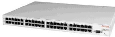
Mid-Span power supply
