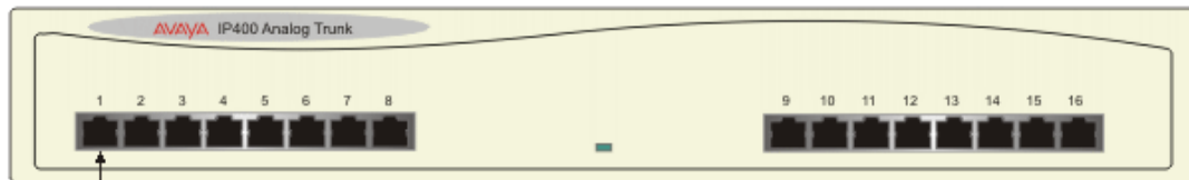
Analog Trunk Ports Individually switchable to loop or ground start.
