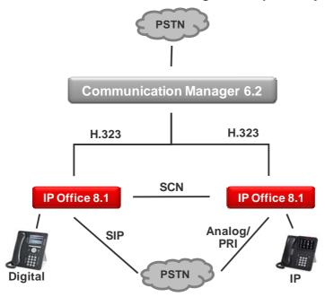
The H323 protocol is used for trunks between the IP Office nodes and the CM. The IP Offices are a network of SCNs and can use the advanced SCN feature set between each other.
