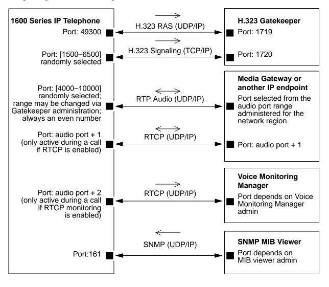
Figure 2: Initialization and Address Resolution Diagram
