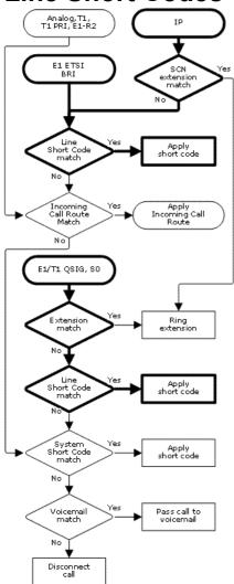
Line short codes are applied to the digits received with incoming call. They are not used with all types of trunk. On other trunks they are only used in particular operation modes. The stage at which they are applied also varies.
