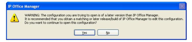
The IP Office Administration installer will detect previous installed versions and upgrade automatically. If a version earlier than 4.2 is installed, this must first be uninstalled before installing 9.0.12.0.1006. It is not necessary to restart the PC after upgrading unless instructed to do so. Before upgrading the IP Office system software ensure a backup of the system configuration exists.
